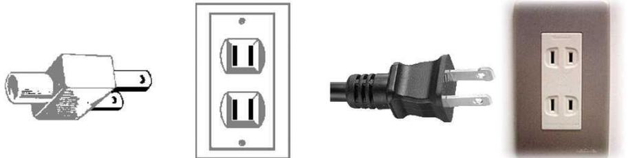
Type B (plug A and C can normally also be used with socket B)
